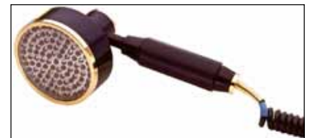
Figure 2. The 104 Diode Cluster Probe (THOR).
